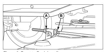
Figure 8. Front to Back Leveling
